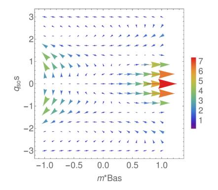
FIG. 3. The magnetization conductance  $\mathbf{G}_L$  (in units of  $\gamma$ ) injected into the left unpolarized lead ( $p_L = 0$ ) due to a full polarization of the right lead ( $p_R = 1$ ), for different values of the SOI and the Zeeman energy on the link, with  $\hat{\mathbf{n}}_R = \hat{\mathbf{b}}$ . The arrows are all in the  $\hat{\mathbf{b}}$ - $\hat{\mathbf{s}}$  plane.
